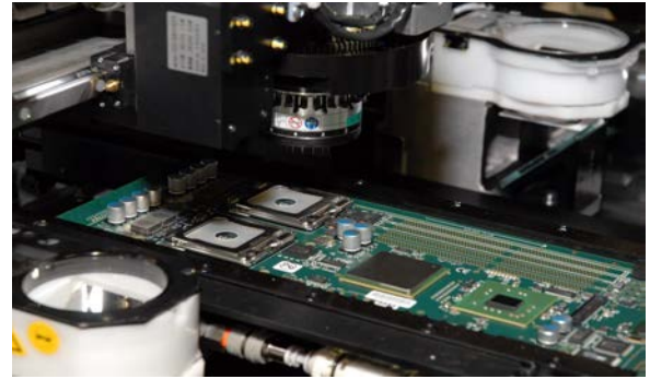
Figure 8 – Inside a Surface Mount Machine at Trenton’s Utica, NY Manufacturing Plant
