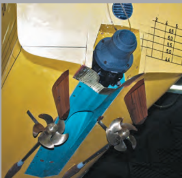
Cutting-edge shipbuilding sciences: streamlined, fast mono-hull with slender forefoot skeg for increased efficiency and reduced yawing (left). CODAG/WARP propulsion system (right)
