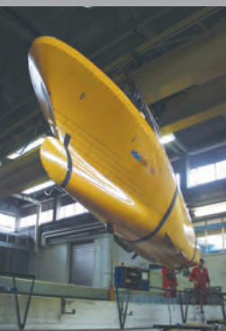
Cutting-edge shipbuilding sciences: streamlined, fast mono-hull with slender forefoot skeg for increased efficiency and reduced yawing (left). CODAG/WARP propulsion system (right)
